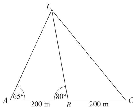
A landmark  $L$  is observed by a surveyor from three points  $A, B$  and  $C$  on a straight horizontal road, where  $AB = BC = 200$  m. Angles  $LAB$  and  $LBA$  are  $65^\circ$  and  $80^\circ$  respectively (see diagram). Calculate
