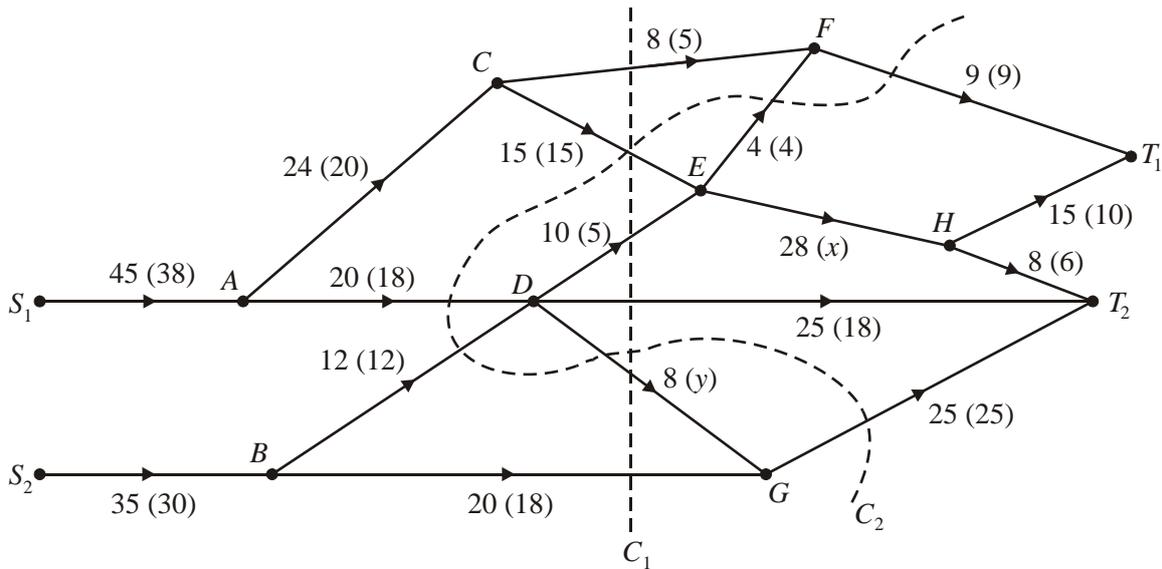
Figure 1 shows a capacitated, directed network. The unbracketed number on each arc indicates the capacity of that arc, and the numbers in brackets show a feasible flow of value 68 through the network.
