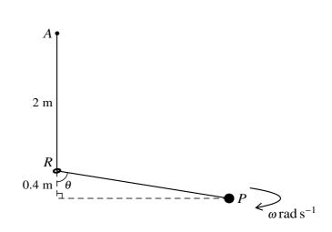
One end of a light elastic string with modulus of elasticity 15 N is attached to a fixed point A which is 2 m vertically above a fixed small smooth ring R. The string has natural length 2 m and it passes through R. The other end of the string is attached to a particle P of mass m kg which moves with constant angular speed  $\omega$  rad s<sup>-1</sup> in a horizontal circle which has its centre 0.4 m vertically below the ring. PR makes an acute angle  $\theta$  with the vertical (see diagram).
