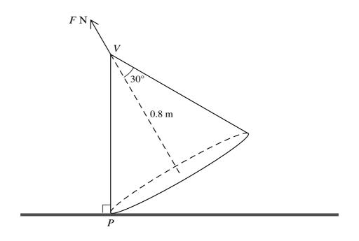
A uniform solid cone with height 0.8 m and semi-vertical angle 30° has weight 20 N. The cone rests in equilibrium with a single point P of its base in contact with a rough horizontal surface, and its vertex V vertically above P. Equilibrium is maintained by a force of magnitude F N acting along the axis of symmetry of the cone and applied to V (see diagram).
